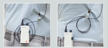
**4)** Always try to keep the cable close to your body or beneath your lab coat. The cable clip can help you to attach the cable as required. Also make sure to keep the cable as short as possible to avoid getting it caught on any equipment. Use the cable holder to coil up the cable. Simply roll it up 2–3 times as seen in the picture:
