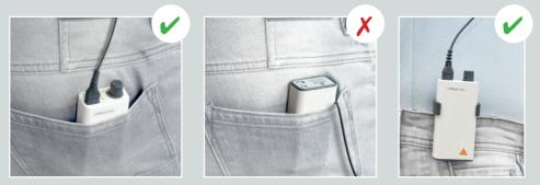
2) Ensure that you put your mPack mini Power Source with the "head up" in your pocket. Wearing the mPack mini bottom down, the cord can not be ripped out of the plug in the battery pack, thus could lead to intensive stretching and bending which leads to breaking or intensive wear & tear.
